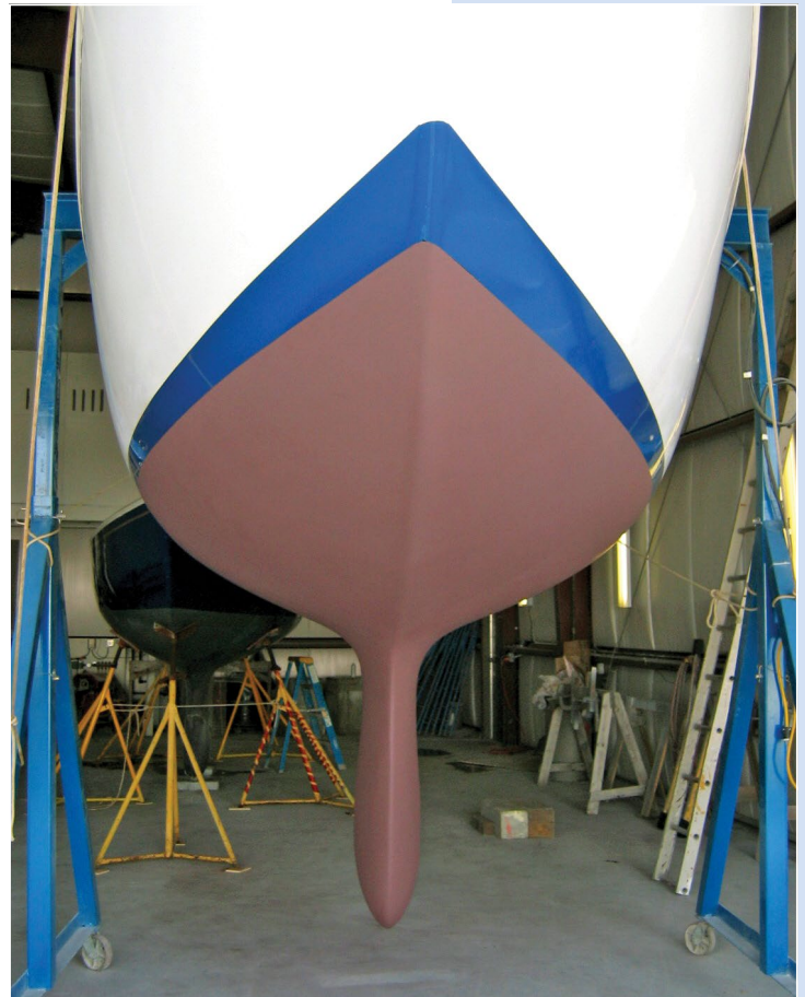
Fresh antifouling paint applied, ready to race.
