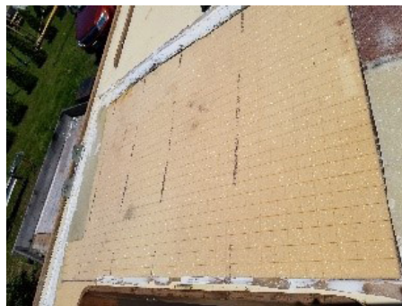
Just Above: Picture 9 Far Left: Picture 10 then Picture 11 bi-axial glass, lots of poly resin, and the new Corecell material, we applied buckets of weights to ensure that the Corecell would bend into the appropriate arch shape. (See picture 10) When we came back to the boat the following weekend, we were surprised and highly disappointed that the deck was “crunchy” and had no
